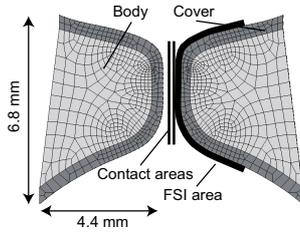
**Figure 1:** Structural FE model with two layers (body and cover), contact areas and fluid-structure interaction (FSI) areas.
