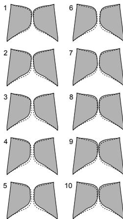
**Figure 4:** One complete oscillation cycle of 5 ms of the structure divided in ten frames.
