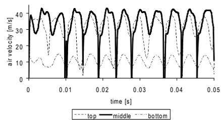
**Figure 6:** Air velocity over time at three nodes according to Fig. 2.
