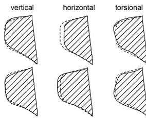
**Figure 3:** First three eigenforms of the structural model. The dashed line marks the original shape of the model while the lined shape shows the two extrema (minimum/maximum) of the eigenform.
