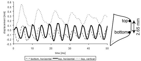
**Figure 5:** Vertical and horizontal displacements of two nodes and their position.
