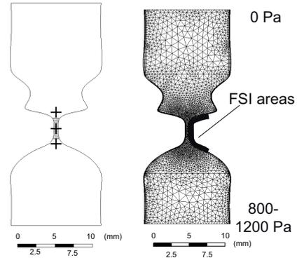
**Figure 2:** Fluid FV model. Left-hand side: Sketch of the fluid model. The striped zone is the zone where the loss coefficient  $K_l$  is introduced when a control distance is undercut. The crosses mark nodes where velocity and pressure is read off for the diagrams and are referred to as “top”, “middle”, and “bottom”. Right-hand side: FV net with FSI areas and pressure boundary conditions.
