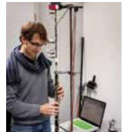
Set-up for musical instrument directivity measurements in the horizontal plane and results (left/centre); set-up for measurement of input impedances of woodwind instruments (right)
