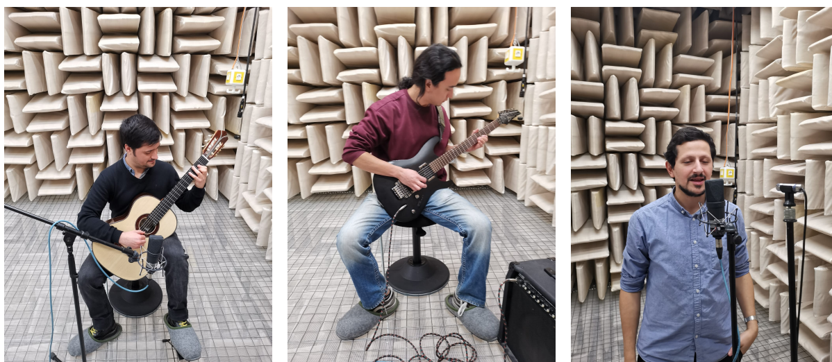
Figure 3.6.: Sound sources recorded in anechoic chamber to use as dry samples.
